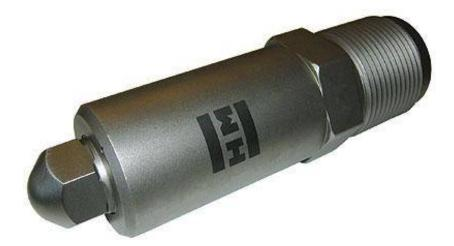
The machine nozzle NM is a valve gate nozzle for injection moulding machines. It is used to stop leaking of material during loading, and upon removal from the moulding machine.
