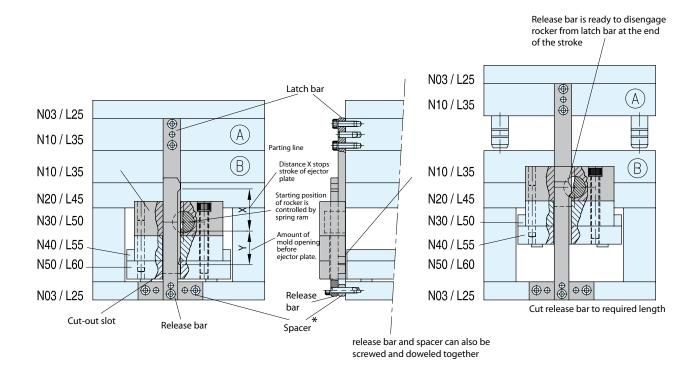
With Latch-lok LL-151 especially the ejector plate is moved, ejector plate (N 50) has to overhang enough, so that body and, if necessary spacer\* could be mounted. Body and spacer are to be screwed and doweled with N 50.
