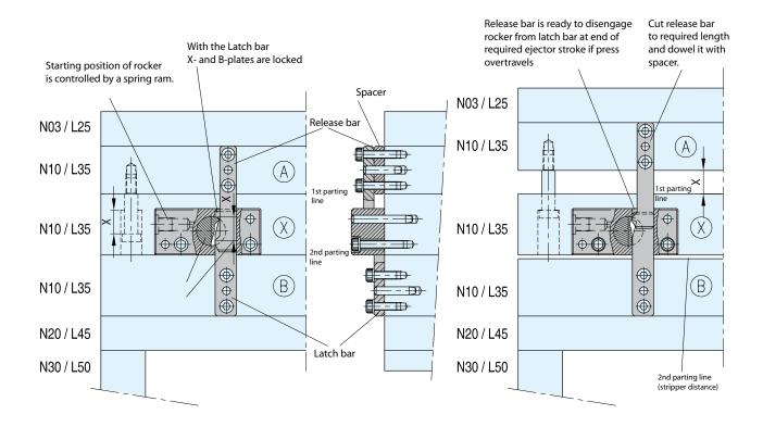
For one mold at least 2 Latch-loks are required, which are respectively mounted at outer surfaces (center of the mold). Body must be parallel screwed and doweled at the molding plate. Latch and release bars must be screwed at 90° to the parting line (Slotted holes facilitate final adjustment). The bars have to slide properly in the body.
