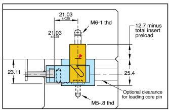
Note: 21.03 dimension must be maintained to ensure proper shut-off.
