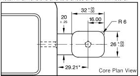
Note: When the core pin is not shutting off on the inner core wall, the distance from the edge of the insert should be 29.02 for the slide carrier to shut off against the core insert.
