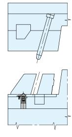
Available in three sizes with increasing weight holding capacities, the Slide Retainers can be used individually or in multiples for larger or heavier slides.
