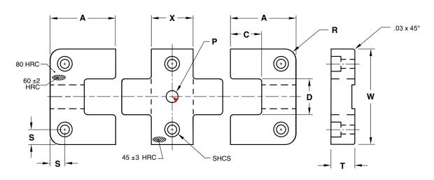
Females (2): M D-2 H Core: 58-62 HRC, Surface: 80 HRC S Titanium Nitride Coated
