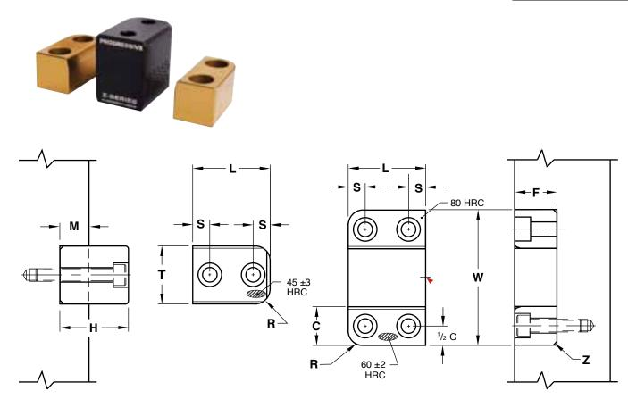
Females (2): M D-2 H Core: 58-62 HRC, Surface: 80 HRC S Titanium Nitride Coated Male: M H-13 H 42-48 HRC S Salt Bath Nitrided
