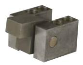
The accelerated knock-outs are simple in design, using a pivot-type motion for accelerated ejection. Mechanical advantage is 2:1. They will accommodate ejector pins up to 9,5mm in diameter. (Pins with head diameters over 15,8mm can be ground down to fit). Simplicity of design permits accelerated knock-outs to be either inserted into the ejector plate (as shown below) or top mounted, depending on space available for the ejection movement.
